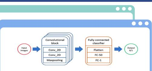
Fig. 5 The Convolutional Neural Network architecture
